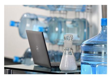
Fifty percent of the matrix for the new semi-finished products consists of recyclates originating from the recycling of reusable polycarbonate water bottles. The primary target application for these products includes laptop covers and housings for smartphones, tablets, e-books, and cellphones. Photo: LANXESS AG
