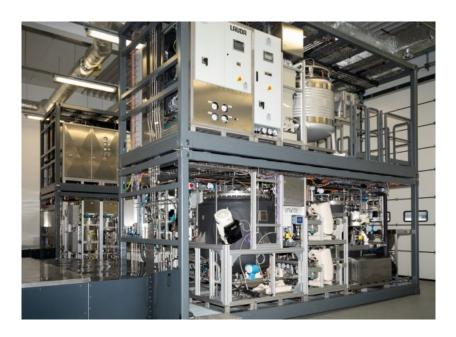
Modular plant for resource-efficient manufacture of leather chemicals. This plant allows tanneries to recycle shavings from leather production directly on-site and use these to produce X-Biomer retanning agents fully automatically. Photo: LANXESS AG
