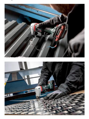
The cordless nibbler is the perfect choice for working corrugated and trapezoidal sheets, and the cordless sheet shears are ideal for cutting flat sheets. The housing shells and the upper and lower shells of the batteries for both tools are made from polyamide 6 Durethan materials from LANXESS. Photos: Metabo
