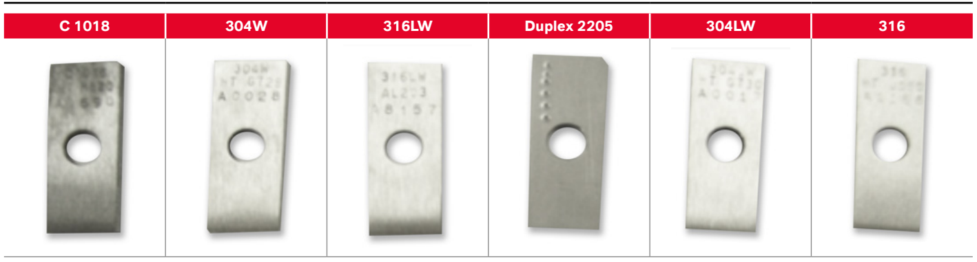
Test coupons after 90-day above surface exposure at 50 °C removed from test bottles (after cleaning)
