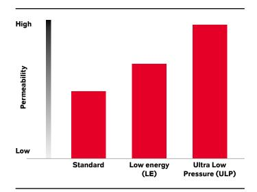
The barrier layers have a lower level of cross-linking than in LE types. ULP elements are available with diameters of 4" or 8" and with membrane surface areas of 7.9 m² or 40.9 m². Their salt rejection under standard conditions is 99.5%.
