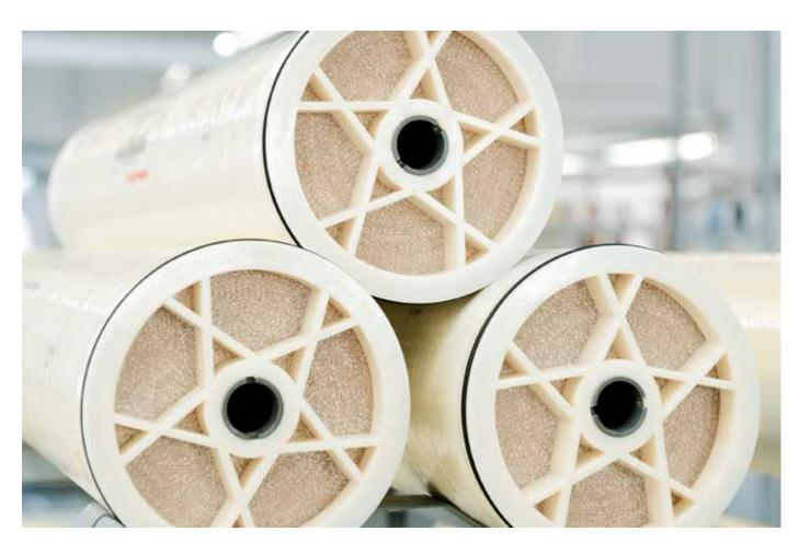
The membranes are based on a three-layer composite structure that is manufactured in several stages. A single Lewabrane® membrane element consists of a bundle with more than 20 membrane layers. This final spiral-wound element is created in a fully automated production process.
