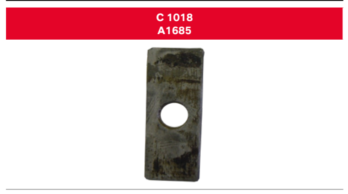
Figure 8: Back side of C1018 coupon after 90-day subsurface exposure at 50°C (before cleaning)
