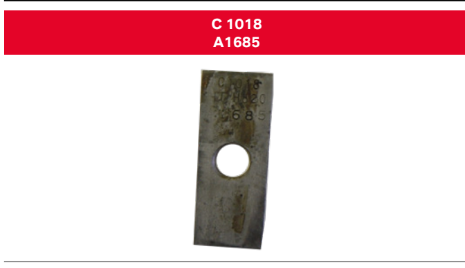
Figure 7: Front side of C1018 coupon after 90-day subsurface exposure at 50°C (before cleaning)
